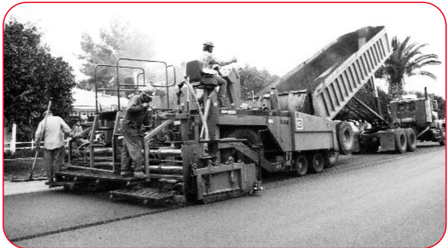
This is a Caterpillar AP-1200. Note the hydraulically extendible screed which adjusted from a paving width of 10 feet to 19 feet and 6 inches. This photo is from 1987.
